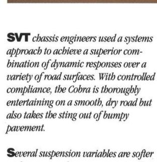
and more compliant to assure that the wide tires maintain consistent contact with the road. In comparison with the Mustang GT, the Cobra's front anti-roll
