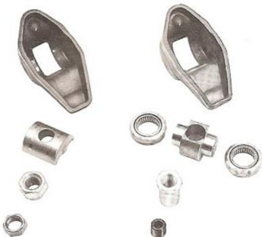
Stock Rocker Arm Assembly On Left. Ford Competition Rocker Arm Assembly (DOZX 6A585-A) On Right.
