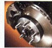
Aluminum twin-piston front calipers reduce unsprung weight and enhance brake pedal feel.
