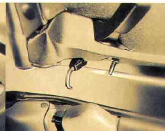
Two easy-to-use latches make retracting the convertible top an effortless task.
