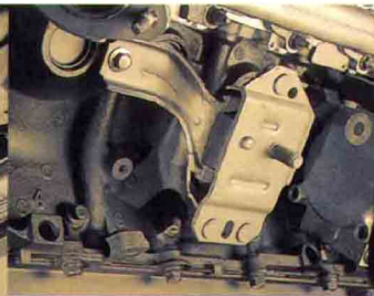
Revised V8 engine mounts provide increased stiffness, reducing mid-vehicle shake, common to convertible vehicles.
