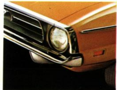
Protection Group guards finish against bumps and scrapes in parking situations. Includes body-side molding with color-keyed vinyl insert and front bumper guards with rubber inserts.
