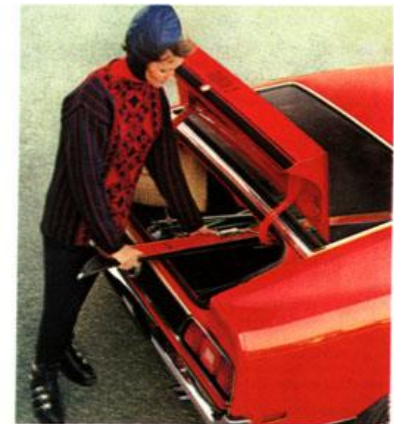
Sport Deck Rear Seat lets you carry bulky or long items in SportsRoof, Mach 1 and Boss 351. Folds flat and permits interior access to trunk. Includes space-saver spare tire.
