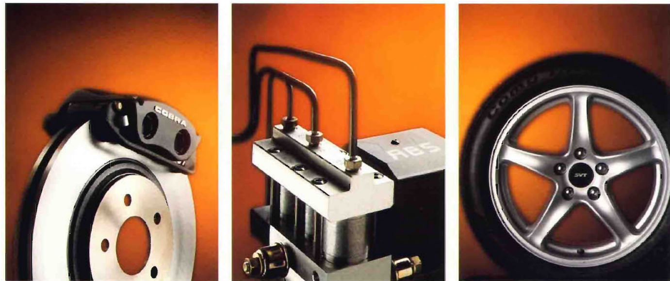
Above, left to right: The Cobra 13.0-inch vented front discs feature curved internal vanes to dissipate heat quickly. The PBR front calipers are a twin-piston design. The Cobra brakes are monitored and controlled by a three-channel, four-sensor ABS system that can modulate and adjust each of the four calipers every 10 milliseconds. The Cobra 17.0-inch five-spoke alloy wheels are wrapped with BFGoodrich Comp T/A ZR radials.
